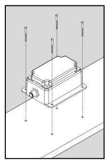
Figure 1 – Mounting the ACM100
